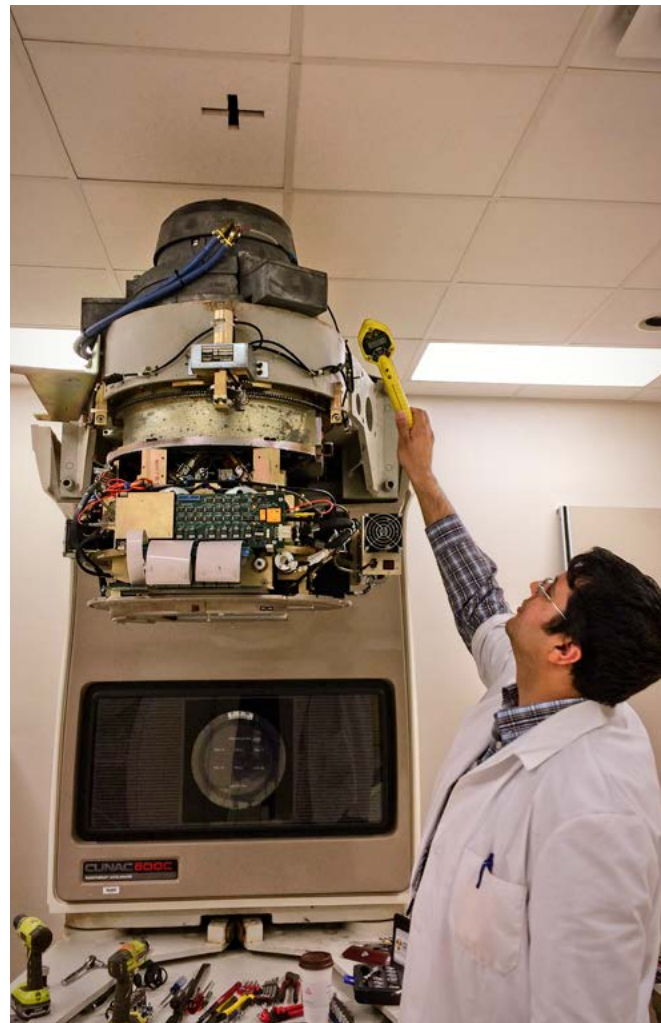
RSO radiation specialist Amin M. Hamideh conducts a survey on the gantry/primary collimator of a decommissioned linear accelerator at the School of Veterinary Medicine.
