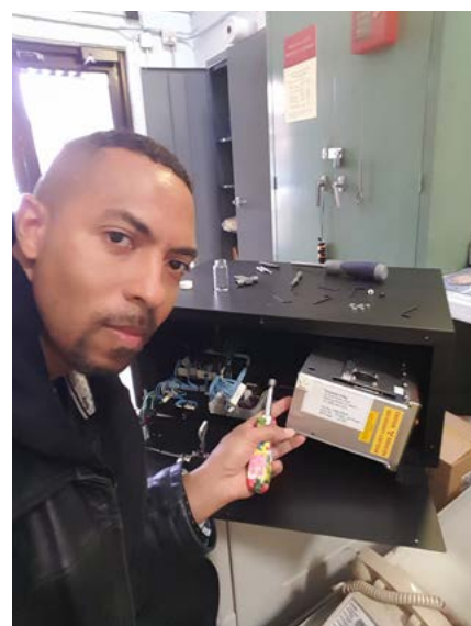
RSO operations manager Jabari Robinson removes an X-ray tube from a Kodak In-vivo Multispectral Imaging System for decommissioning. This system was used for in-vivo imaging of small animals for drug development and life science research.
