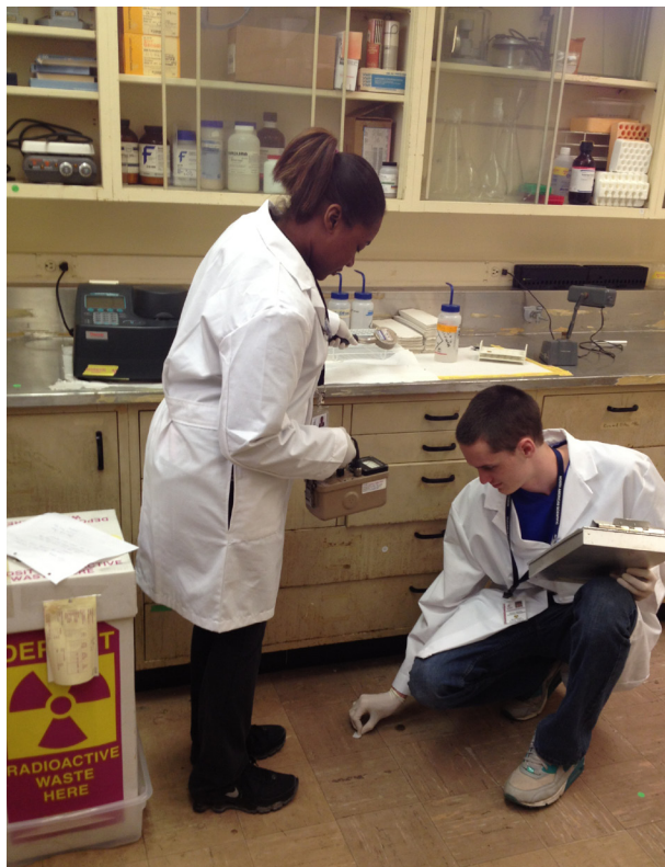
RSO technical assistants Jerrica Williams (left) and Dylan Albers carry out a routine radiation laboratory contamination survey using a pancake Geiger-Mueller probe survey meter and smears.
